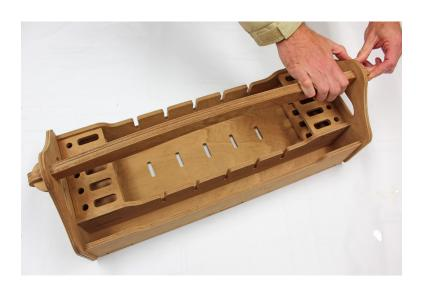
... and push the second key through the hole in the handle. You may have to bend the top of the end panel inwards a bit to get the key to slide into place, or gently tap the key with a rubber mallet.
